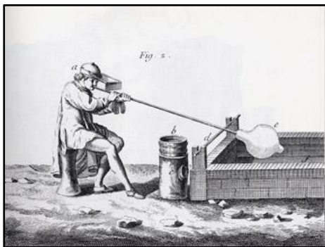
A globe is formed at the end of a blowpipe
